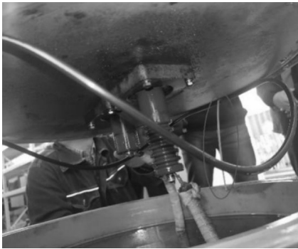
图3 密封圈处存在尼龙扎带 Fig. 3 Nylon tape at the sealing ring
